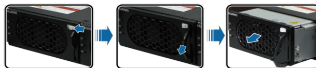
Figure 5 Removing the old rectifier
