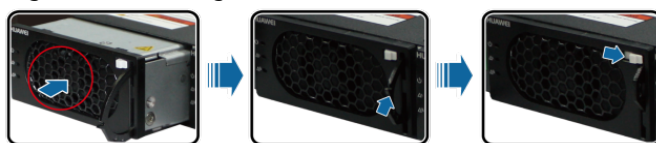
Figure 6 Installing the new rectifier
