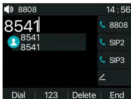
Picture 13 - Enable voice channel dialing
