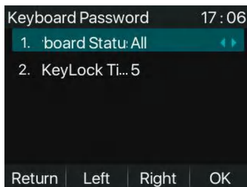
Picture 117 - Set keyboard lock password
