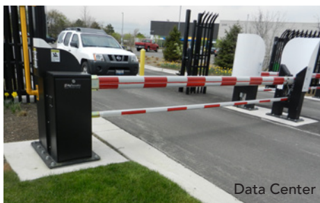
StrongArm M30 ASTM F2656-07 M50-P1* 6 to 8 seconds Open/Close time 12 to 24 ft clear opening
